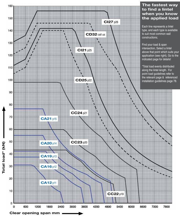
Lintel standard lengths are 150mm increments (grid spacing) starting at 450mm
